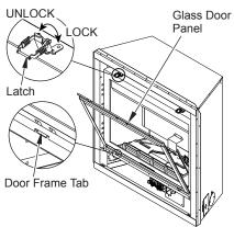
Figure 45 - Removing/Replacing Glass Door
